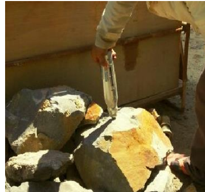
Figure 4 Rebound Hammer Test
